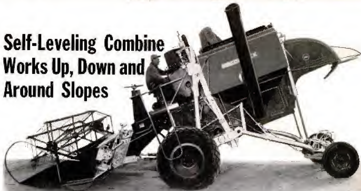
A self-leveling combine in position for downhill work. The driver's seat is reversed for this operation. Idaho Machine and Sheet Metal Works photo.
